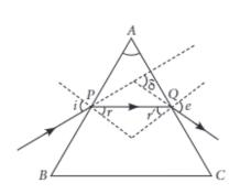
The incident ray suffers a deviation or bending through an angle  $\delta$  due to the refraction through prism. This angle is called angle of deviation as shown in figure.
