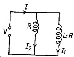
$R_{eff}$  is the impedance of the coil & the resistance in parallel.
