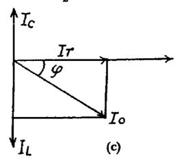
4.145 When the coil and the condenser are in parallel, the equation is
