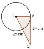
Now,  $\triangle OPQ$  is a right-angled triangle at P as  $OP \perp PQ$ [Tangent through a point on the circle is perpendicular to the radius through point of contact] By Pythagoras theorem, we have  $OP^2 + PQ^2 = OQ^2$  $\Rightarrow OP^2 + 24^2 = 25^2$  $\Rightarrow OP^2 + 576 = 625$  $\Rightarrow OP^2 = 625 - 576 = 49$  $\Rightarrow OP = 7 \text{ cm}$
