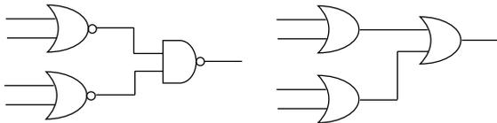
So output of 1<sup>st</sup> NOR-NAND structure  $= A + B + C + A$
