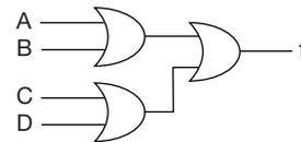
Each 2 input OR gate required 3-2 input NAND gates
