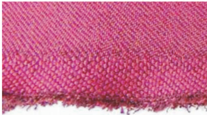
Fig 31: Selvedge in a woven fabric
