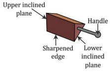
The upper part of the wedge has a large area and the lower sharpened edge has very less area. On hammering, a large pressure on the sharp edge is created than on the upper part. A wedge is used for splitting logs. The thinner the wedge, the easier it is to drive it into a log. A speed boat has its leading edge shaped like a wedge to cut through water easily.
