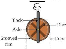
On pulling one end of the rope down, the object tied to the other end of the rope is lifted. Thus, the direction of force can be changed.
