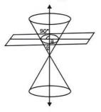
(ii) When  $\theta < \alpha < 90^\circ$ , then cutting plane section is an ellipse.
