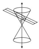
(iii) When  $\alpha=\theta$  i.e., plane is parallel to a generator, then cutting plane is parabola.
