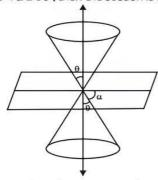
(ii) When  $\theta = \alpha$ , then the plane contains the generator of cone and the section is a straight line. It is a degenerated case of a parabola.
