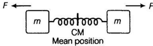
The system is divided into two similar systems with spring divided in two equal halves, forming spring constant
