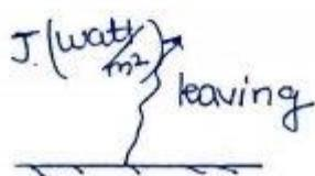
The total thermal radiation leaving a surface per unit time per unit area is known as Radiosity ( $J$ )
