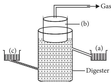
The diagram above is that of a typical biogas plant. Explain the sequence of events occurring in a biogas plant. Identify a, b and c.
