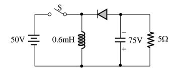
The capacitor is large enough so that the ripple across it is negligible and at steady state acquires a voltage as shown. The peak current in amperes drawn from the 50 V DC source is \_\_\_\_\_. (Give the answer up to one decimal place.)
