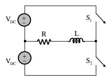
The switch control signal of the converter are generated using sinusoidal pulse width modulation with modulation index, M = 0.6. At 50 Hz, the RL-load draws an active power of 1.44 kW. The value of DC source voltage  $V_{DC}$  in volts is
