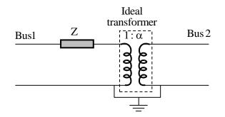
For the given circuit,  $Y_{bus}$  and  $Z_{bus}$  are bus admittance matrix and bus impedance matrix,
