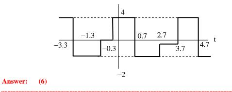
22. The mean square value of the given periodic waveform f(t) is
