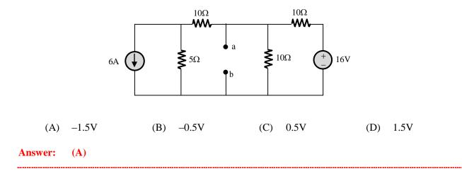
**29.** For the network given in figure below, the Thevenin's voltage  $V_{ab}$  is
