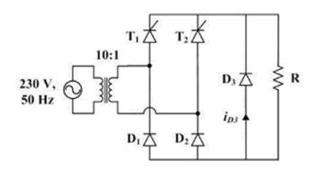
Assume that all devices are ideal. The firing angles of the thyristors  $T_1$  and  $T_2$  are 90° and 270°, respectively. The RMS value of the current through diode  $D_3$  in amperes is \_\_\_\_\_.
