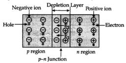
Applying forward bias, the depletion region reduces and again electrons can diffuse.
