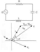
From the phasor relation, voltages  $V_L + V_R + V_C = V$ , as  $V_C$  and  $V_L$  are along the same line and in opposite directions, so they will combine in single phasor ( $V_C + V_L$ ) having magnitude  $|V_{Cm} - VLm|$ . Since voltage V is shown as the hypotenuse of right-angled triangle with sides as  $V_R$  and ( $V_C + V_L$ ), so the Pythagoras Theorem results as :
