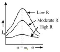
The Q -factor of the series resonant circuit is defined as the ratio of the voltage developed across the capacitance or inductance at resonance to the impressed voltage which is the voltage applied.
