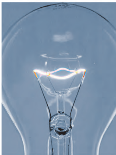
Fig. 14.12 Glowing filament of an electric bulb (incandescent)
