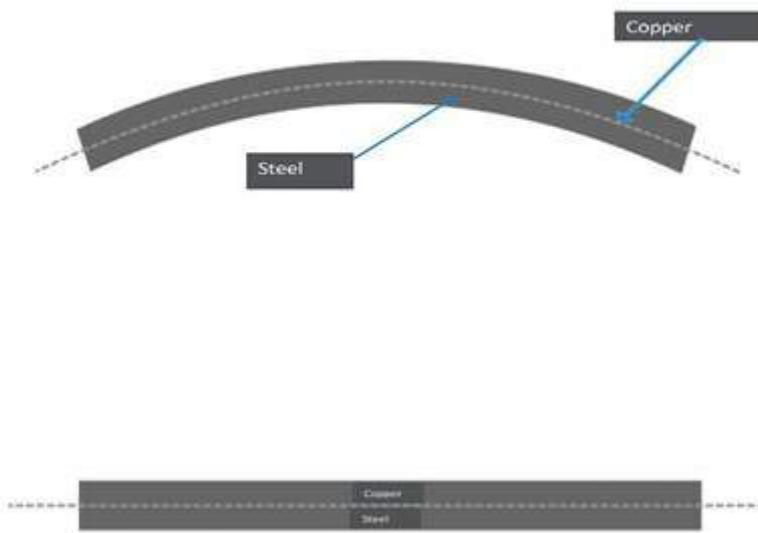
Linear expansion coefficient of copper is greater than the steel ( $\alpha_{\text{copper}} > \alpha_{\text{steel}}$ ). So, on heating copper gets more expansion than steel. So the bimetallic strip will bend with the copper on the convex side.
