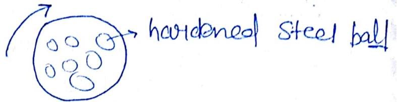
If the material is extremely brittle we can directly put into the drum and when there is little bit ductility. Initially it will be dipped in liquid nitrogen and placed in drum. By the repeated collision between the material and steel ball material will convert in nanoparticles but it is a time consuming process.
