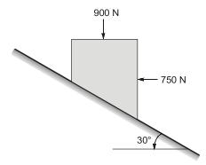
The coefficient of static friction between the block and surface is \_\_\_\_\_ (round off to two decimal places)
