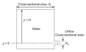
Neglecting any losses, the time taken by water in the tank to reach a level of y = H/4 is \_\_\_\_\_ seconds (round off to one decimal place).
