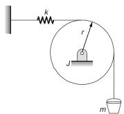
The pulley radius is r and its mass moment of inertia is J. Assume that the mass is vibrating harmonically about its static equilibrium position. The natural frequency of the system is
