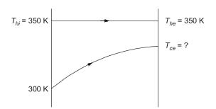
$$NTU = \frac{UA}{(\dot{m}c_p)_{\text{small}}} = \frac{1500 \times 400}{100 \times 4000} = 1.5$$
