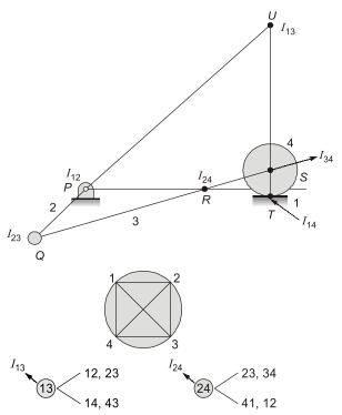
Points P, Q, R, S, T and U are instantaneous centers of mechanism.
