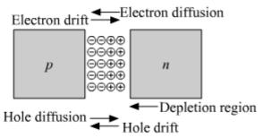
The positive ions and negative ions develops potential difference across the junction and an internal electric field E, directed from n-side top-side. The potential difference gets developed due to positive and negative ions across the depletion layer is called the **potential barrier**. It stops the diffusion process. This potential barrier reduces in forward biased mode and increases in reverse biased mode.
