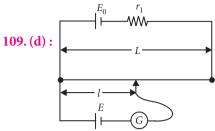
The current through the potentiometer wire is  $I = \frac{E_0}{(r+r_1)}$  and the potential difference across the wire is
