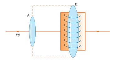
The inconsistency may disappear if displacement current is included between the plates. So generalised Ampere's circuital law can be given as
