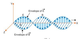
(b) The speed of electromagnetic wave  $|c| = \frac{|E_0|}{|B_0|}$
