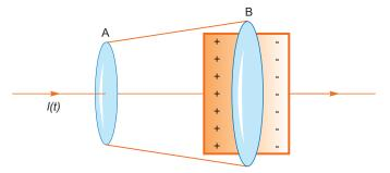
Now we consider a pot like surface enclosing the positively charged plate and nowhere touches the conducting wire,
