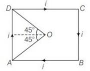
Let O be the centre of square ABCD of side 2a carrying current i ampere. The magnetic field due to infinite length of
