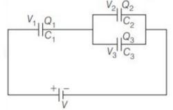
According to Kirchhoff's first law,  $Q_1 = Q_2 + Q_3$ As  $C_2$  and  $C_3$  are in parallel,  $V_2 = V_3$  and according to Kirchhoff's second law  $V = V_1 + V_2 = V_1 + V_3$
