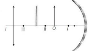
As a real and inverted image of O is obtained by concave mirror.  $\therefore$  I must be the focal point. And hence, II must be the centre of curvature.
