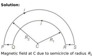
$B_{1} = \frac{\mu_{0}I}{4R_{1}}$  [outside of paper]  $B_{2} = \frac{\mu_{0}I}{4R_{2}}$  [inside of paper]
