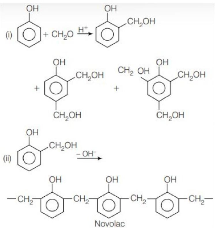
**Step II** On heating above structure, it gives network of phenol and formaldehyde, also known as bakelite.
