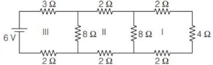
Equivalent resistance of loop I, = 2 + 4 + 3 = 8Ω  $R_{eq} = \frac{R_1 \times R_2}{R_1 + R_2} = \frac{8 \times 8}{8 + 8} = \frac{8 \times 8}{16}$ = 4Ω Equivalent resistance of loop II, = 2 + 4 + 2 = 8Ω  $R'_{eq} = \frac{R_1 \times R_2}{R_1 + R_2} = \frac{8 \times 8}{8 + 8}$ = 4Ω Equivalent resistance loop III, = 3 + 2 + 4 = 9Ω Maximum current, i =  $\frac{6}{9} = \frac{2}{3}A$ = 0.66A
