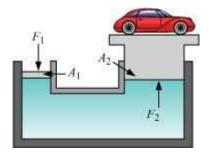
• Therefore, a large force is experienced in the larger cross-section if a smaller force is applied in the smaller cross-section.
