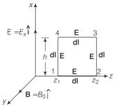
During the propagation of electromagnetic wave a long *z*-axis, let electric field vector (**E**) be along *x*-axis and magnetic field vector **B** along *y*-axis, *i.e.*,  $\mathbf{E} = E_0 \hat{\mathbf{j}}$  and  $\mathbf{B} = B_0 \hat{\mathbf{j}}$ .
