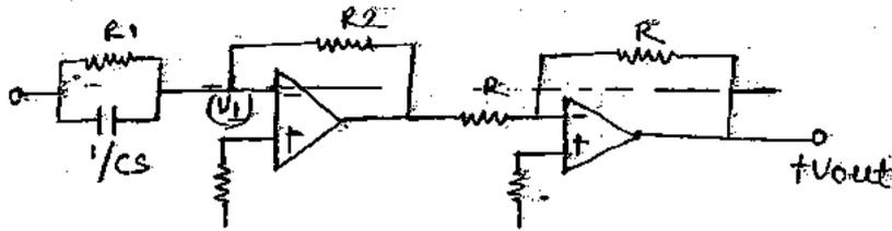
$$\frac{V_e - V_1}{\frac{R_1}{R_1 s + 1}} = \frac{V_1 - V_{out}}{R_2}$$
