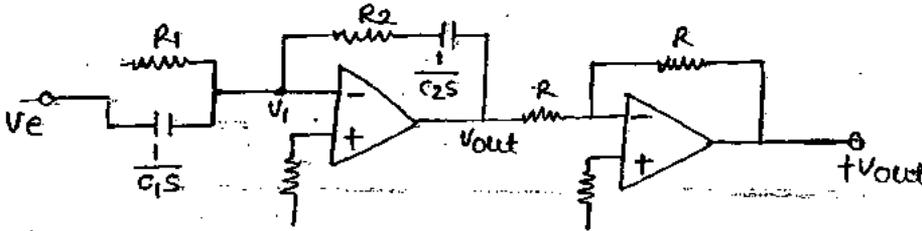
$$\Rightarrow \frac{V_e - V_1}{\frac{R_1}{R_1 C_1 s + 1}} = \frac{V_1 - V_{out}}{\frac{R_2 C_2 s + 1}{C_2 s}}$$
