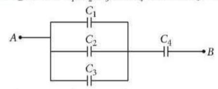
$$\therefore \frac{1}{C_{AB}} = \frac{1}{C_1 + C_2 + C_3} + \frac{1}{C_4}$$
