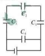
All the capacitors in branch 1 is in series so the charge on each capacitor is  $Q' = \frac{6}{11}CV$
