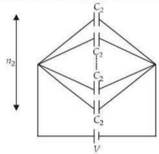
Total capacitance of the parallel combination of capacitors is
