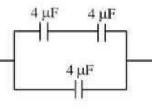
$$C_{\text{eq}} = \frac{4 \times 4}{4 + 4} + 4 = 2 + 4 = 6 \,\mu\text{F}.$$
