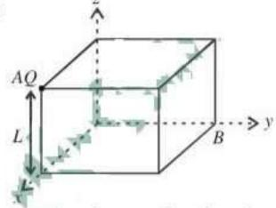
As at a corner, 8 cubes can be placed symmetrically, flux linked with each cube (due to a charge Q at the corner) will be  $\frac{Q}{8\varepsilon}$ .
