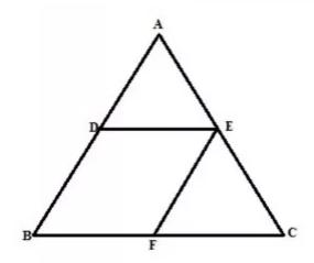
From figure since E is the midpoint of AC and EF||AB Therefore F is the midpoint of BC and 2DE=BC or DE=BF Again D and E are midpoint ,therefore DE||BF and EF=BD Hence BDEF is a parallelogram.
