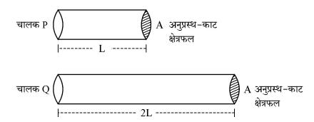
In two conductors of same metal P and Q shown in figure which has more resistance? 1
