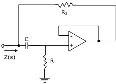
12. Find the value of R' in the circuit of Fig.12 for generating sinusoidal oscillations. Find the frequency of oscillations.
