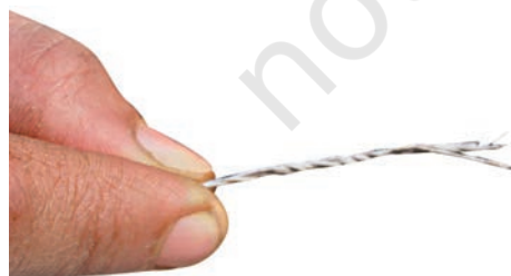
Fig. 3.5 Yarn split up into thin strands
