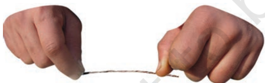
Fig.3.4 Splitting the yarn into thin strands
