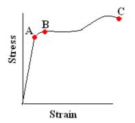
In the region from O to A, the curve is linear. The strain is directly proportional to the stress. Beyond the point A, known as the proportional limit, the relation between stress and strain is not linear.
