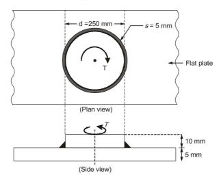
Throat thickness,  $t_t = 0.75 = 0.7 \times 5 = 3.5 \text{ mm}$
