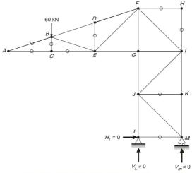
Force in members AB, AC, BC, CE, DE, FH, HI, JK and LM are zero. Hence,  $F_{J\!K}=0; \quad F_{BC}=0; \quad F_{F\!I}\neq 0; \quad F_{E\!G}\neq 0$  Hence, the correct options are (a) and (d).
