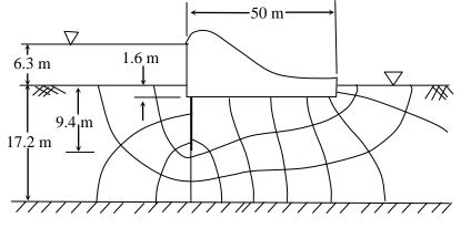
**40.** The flow net constructed for the dam is shown in the figure below.
