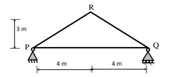
The magnitude of vertical displacement of joint R (in mm) is \_\_\_\_\_
