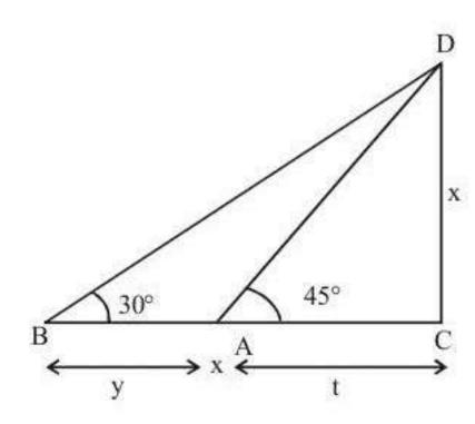
Let CD be a tower of height x metre. Also  $\angle DAC = 45^{\circ}$  and  $\angle DBC = 30^{\circ}$
