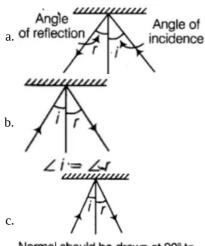
Normal should be drawn at 90° to the reflecting surface of a mirror.
