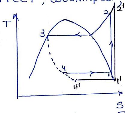
→ The evaporator pressure depends on the temp. of the evaporator, which depends on the desired effect of the machine. (i.e. Air conditioning or ice making)
