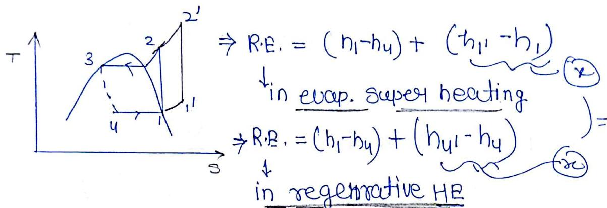
\* In both the cases the ~~same~~ R.E., work input and hence COP comes out to be same but the increased refrigeration effect is obtained at a lower temp. in regenerative H.E.
