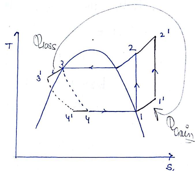
$$\therefore Q_{\text{lost}} = Q_{\text{gain}} \quad R.P = (h_1 - h_4) + (h_4 - h_{4'})$$
