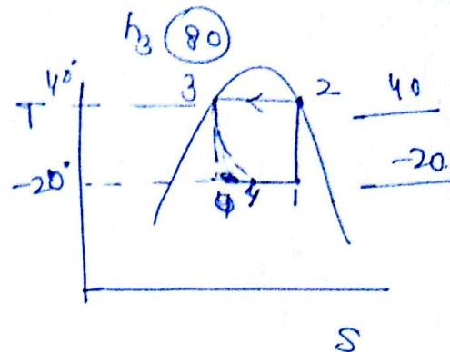
$$\text{COP} = \frac{h_1 - h_3}{h_2 - h_1} = \frac{180 - 80}{200 - 180} = 5$$
