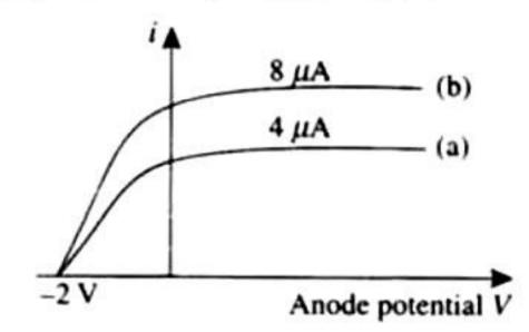
Therefore, the stopping potential is 2V. Saturation current depends on the intensity of light incident. When the intensity is doubled the saturation current will also become twofold. The corresponding graphs are shown in the above figure.
