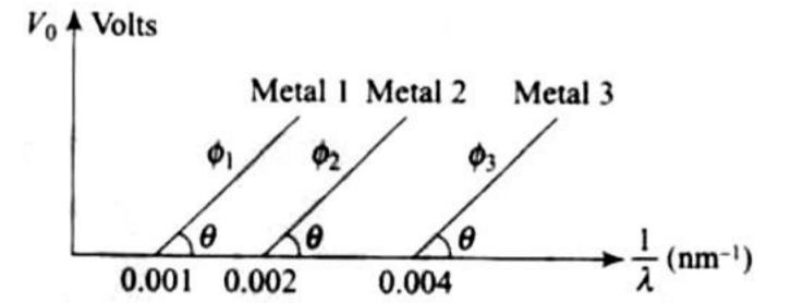
$$V_{0_1}: V_{0_2}: V_{0_3} = 0.001:0.002:0.004 = 1:2:4$$
