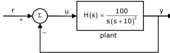
50. The gain margin of the system under closed loop unity negative feedback is
