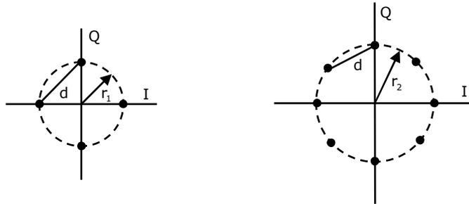
54. For the constraint that the minimum distance between pairs of signal points be  $d$  for both constellations, the radii  $r_1$ , and  $r_2$  of the circles are
