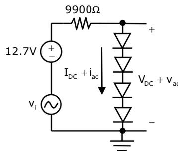
52. The bias current  $I_{DC}$  through the diodes is
