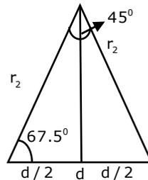
55. Assuming high SNR and that all signals are equally probable, the additional average transmitted signal energy required by the 8-PSK signal to achieve the same error probability as the 4-PSK signal is
