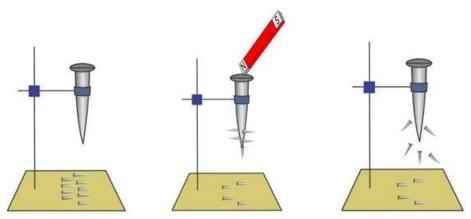
Spread some iron pins on the base of a stand. These pins are not attracted to the nail. When a magnet is touched to the head of the nail, some pins at the base of the stand cling to the nail. This is because the nail turns into a magnet, and hence, acquires the property of magnetism. This is magnetic induction.
