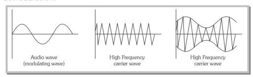
Amplitude modulation (Amplitude of carrier wave modifies in accordance with the amplitude of modulating wave)
