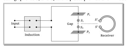
When a high voltage is applied across metallic plates these plates get discharged by sparking across the narrow gap. The spark will give rise to oscillations which in turn send out electromagnetic waves. Frequency of these wave is given by  $v = \frac{1}{2\pi\sqrt{IC}}$
