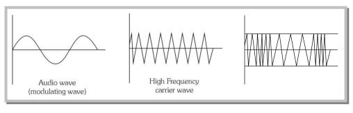
Frequency modulation (frequency of carrier wave changes in accordance with the amplitude of modulating wave)
