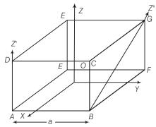
(a) The moment of inertia of cube about z-axis is  $I_z = I_x + I_y$
