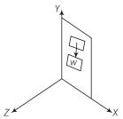
A force can produce torque only along a direction normal to itself as  $\tau = \mathbf{r} \times \mathbf{F}$ . So, when the door is in the *xy*-plane, the torque produced by gravity can only be along  $\pm z$  direction, never about an axis passing through *y*-direction.
