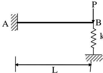
The steel strip is 5mm wide and 10mm thick. A vertical load,  $P = 50 \text{ N}$  is applied at B, as shown in the figure. Considering  $E = 200 \text{ GPa}$ , the force (in N) developed in the spring is \_\_\_\_\_.
