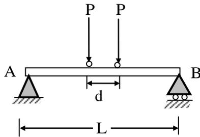
Each wheel transmits a load,  $P = 3 \text{ kN}$  and may occupy any position along the beam. If the beam is an I-section having section modulus,  $S = 16.2 \text{ cm}^3$ , the maximum bending stress (in GPa) due to the wheel loads is \_\_\_\_\_.
