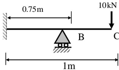
The distance of the point of contraflexure from end A (in m) is \_\_\_\_\_.
