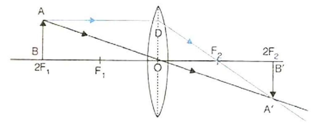
(d) When the object (AB) is situated between  $2F_1$  and  $F_1$ , the position of image (A'B') is beyond  $2F_2$ , it is magnified in size and real and inverted.
