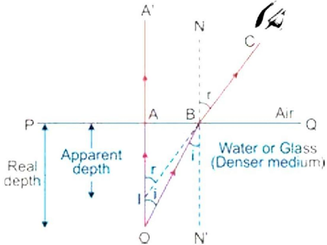
(b) Refractive index of the glass block,  $\mu_g$  = 1.5 Shift in the image = 7mm or 0.7 cm Thickness of glass block or real depth = ?
