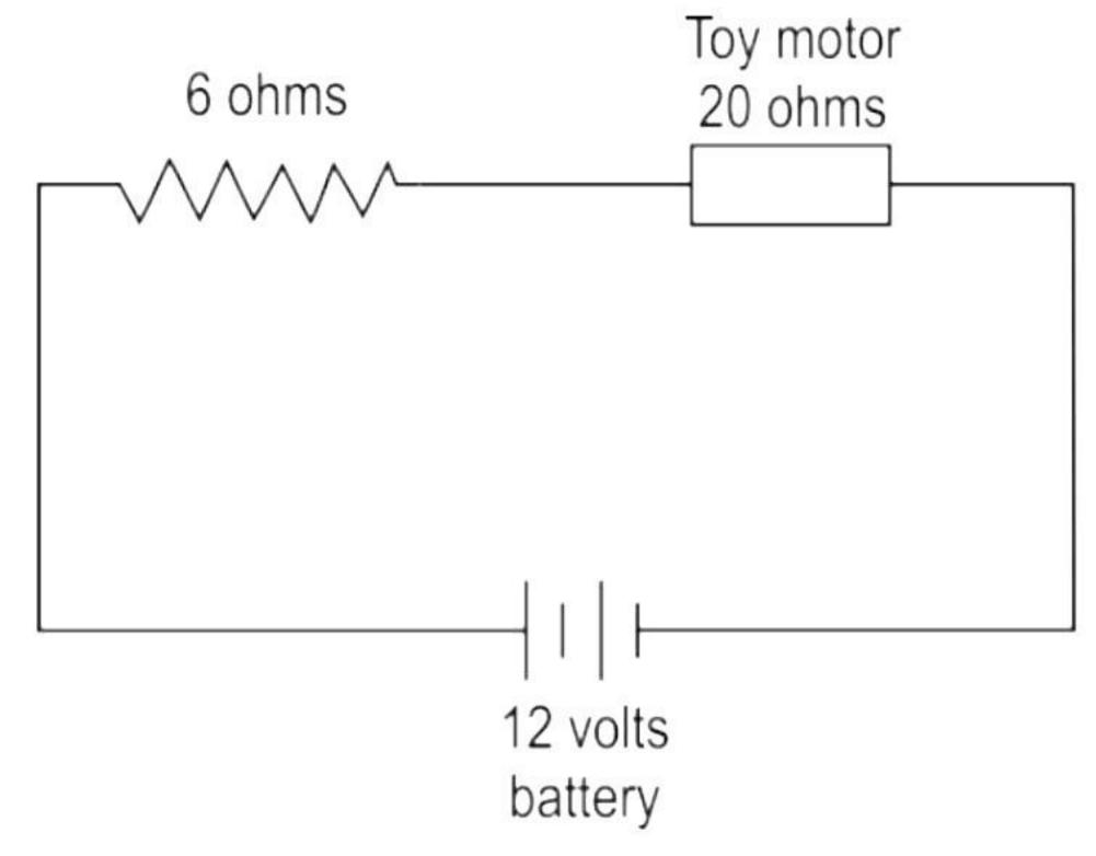
Total resistance of the circuit is  $R_t = 6 + 20 = 26 \Omega$
