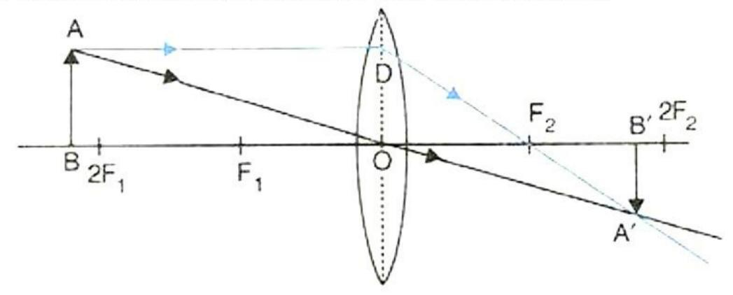
(c) When the object (AB) is situated at  $2F_1$ , the position of image (A'B') is at  $2F_2$ , it is of same size as the object and real and inverted.
