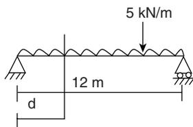
Critical section for shear is at a distance 'd' from support
