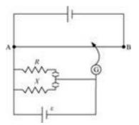
Ans. Resistance of the standard resistor,  $R = 10.0 \ \Omega$ Balance point for this resistance,  $l_1 = 58.3 \ cm$ Current in the potentiometer wire = iHence, potential drop across R,  $E_1 = iR$ Resistance of the unknown resistor = XBalance point for this resistor,  $l_2 = 68.5 \ cm$ Hence, potential drop across X,  $E_2 = iX$
