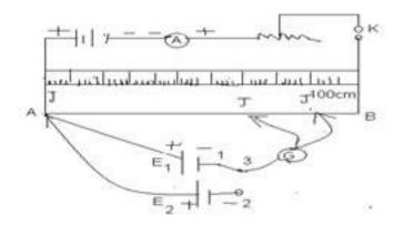
(Condition – close the switch and 3 such that  $E_1$  comes in the circuit)
