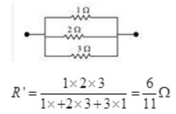
(c) (i) It can be observed form the given circuit that in the first small loop, two resistors of
