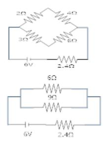
$^{2}\Omega$  and  $^{4}\Omega$  are in series  $^{3}\Omega$  and  $^{6}\Omega$  are in series
