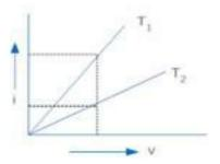
= Smaller the slope larger is the resistance and since resistance increases with the increases in temperature for metals. Slope is small for  $T_2$
