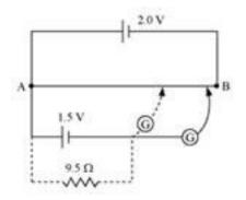
An external resistance (*R*) is connected to the circuit with  $R = 9.5\Omega$
