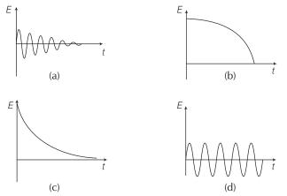
Ans. (c) When a pendulum oscillates in air, it will lose energy continuously in overcoming resistance due to air. Therefore, total mechanical energy of the pendulum decreases continuously with time.
