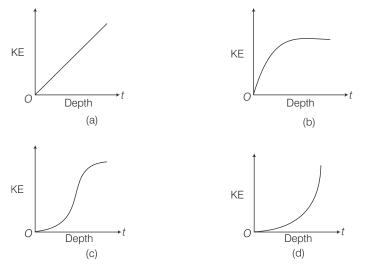
Ans. (b) First velocity of the iron sphere increases and after sometime becomes constant, called terminal velocity. Hence, accordingly first KE increases and then becomes constant which is best represented by (b).
