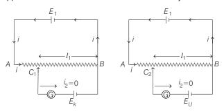
We calibrate the device by replacing  $E_2$  by a source of known emf  $E_k$  and then by unknown emf  $E_u$ . Let the null points are obtained at lengths  $l_1$  and  $l_2$ .
