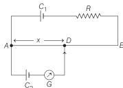
Statement II At the balance point, the potential difference between AD due to cell  $C_1 = E_2$ , the emf of cell  $C_2$ .
