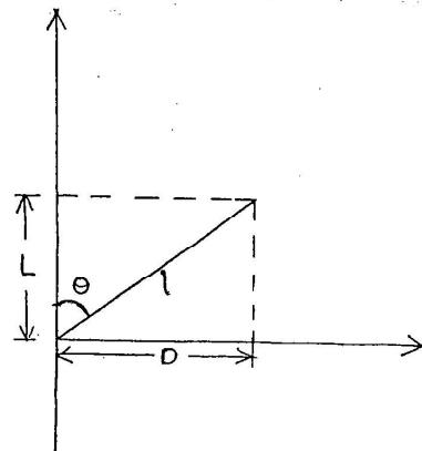
Meridian distance of a line is defined as the meridian distance of its midpoint.
