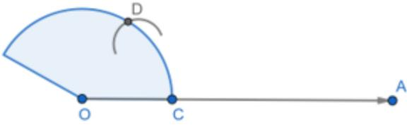
Step 4: With D as center and the same radius, draw an arc cutting the arc cutting at E.
