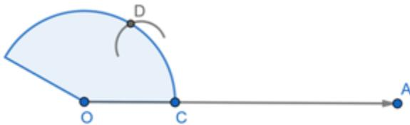
Step 4: With C and D as centres, and any convenient radius (more than  $\frac{1}{2}$  CD), draw two arcs intersecting at B. join OB. Then  $\angle AOB = 30^\circ$
