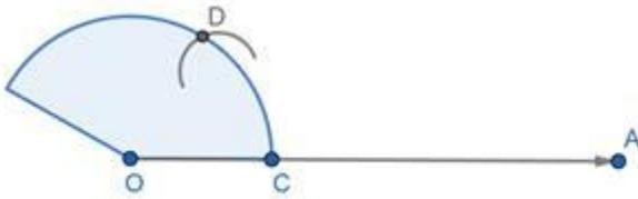
Step 4: With D as center and the same radius, draw an arc cutting the arc cutting at E.
