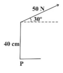
The magnitude of force is  $|\vec{F}| = 50$  N And magnitude of position vector is  $|\vec{r}| = 40$  cm = 0.4 m Then magnitude of torque about P is:  $|\vec{\tau}| = |\vec{F}| |\vec{r}| \sin \theta$ Here  $\theta = 90^{\circ} - 30^{\circ} = 60^{\circ}$ Then  $|\vec{\tau}| = (50)(0.4) \sin 60^{\circ}$ = [17.3 J]
