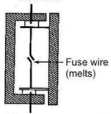
When excess current flows fuse wire melts and breaks
